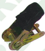
R1005 1" Ratchet Buckle, Rubber Hand, 25mm B/S: 800Kgs/ 1760Lbs
